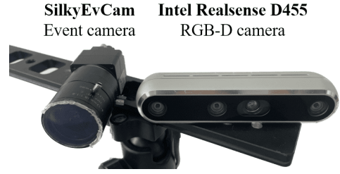
Fig. 6. Illustration of the stereo event-intensity camera setup. It features a SilkyEvCam event camera (left) and an Intel Realsense D455 RGB-D camera (right). Both cameras are synchronized with a baseline of 8cm.
